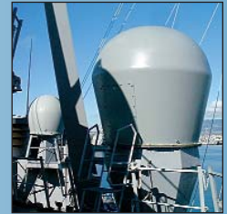
8-ft. (2.4m) radome – shipboard communications
