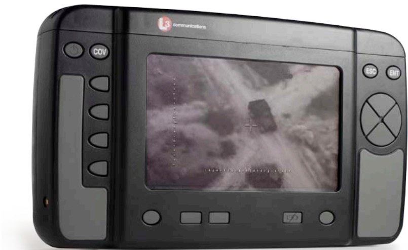
In 2008, L-3 began delivery of the ROVER 5, the next generation of its highly successful Remote Operated Video Enhanced Receiver (ROVER) product line. ROVER 5 transmits and receives live video and other data to and from UAVs, gunships and fighter aircraft for enhanced ground force situational awareness.
