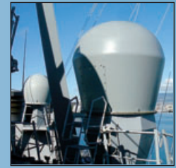
8-ft. (2.4 m) radome – shipboard communications
