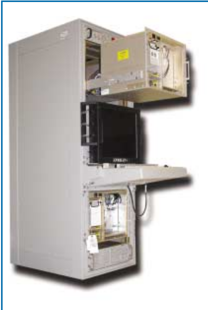
Standard Navy rack upgraded with 2 RCCS Universal Processor Chassis and 1 RCCS Rugged 20-inch Flat Panel Display
