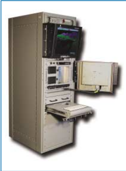
Standard Navy rack upgraded with 2 RCCS Universal Processor Chassis and 2 RCCS Rugged 20-inch Flat Panel Display
