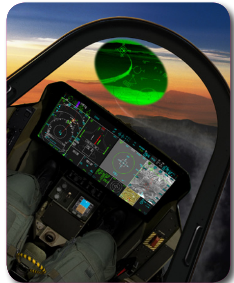
The Large Area Avionics Display installed in the F-35 Lightning II
