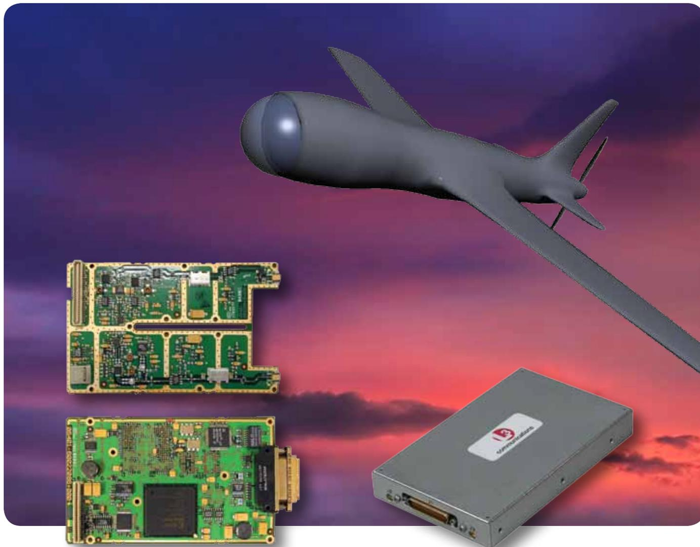
The L-3 Communications' Mini UAV Data Link is a small, lightweight, affordable, modular and scalable data link that enhances a mini UAV's security and range. L-3's Mini UAV Data Link provides guaranteed UAV control, high quality MPEG-4/MPEG-2 or other format video transmission, data security, flexible data types and adaptive data rates with flexible bandwidths for extended range. The low size, weight and power is a perfect fit for UAVs with wing spans as small as 24 to 36 inches.
