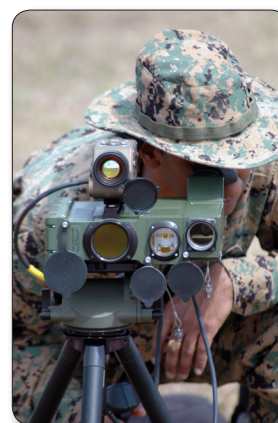
Laser Designator/Range-Finder, Direct View-Optics Module
