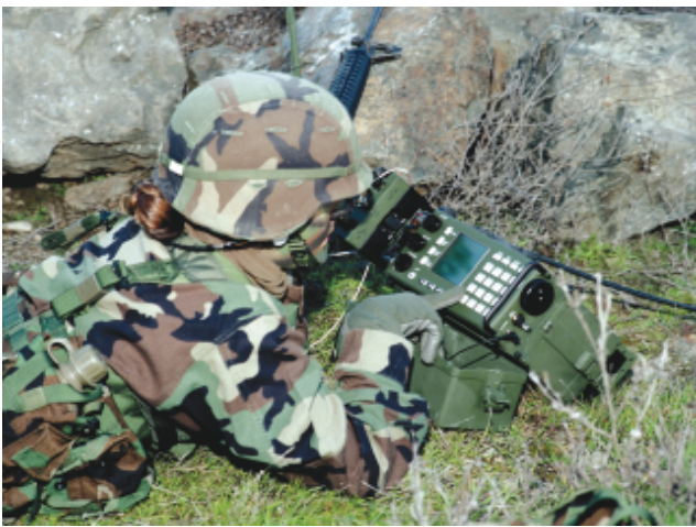
THE MD-405A RECEIVER/PROCESSOR IS THE HEART OF THE AN/PRD-13(V)2 SYSTEM.
