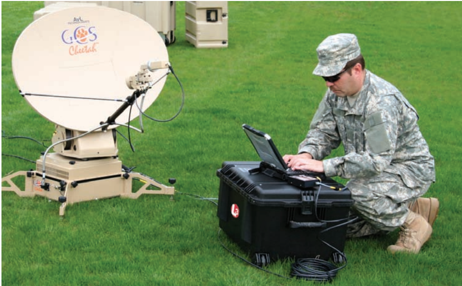
The L-3 Cheetah is an auto-acquire flyaway VSAT system currently used in-theater to support the U.S. military. It provides secure connectivity for voice, data and video broadcast or conferencing and is capable of T1 data rates.
