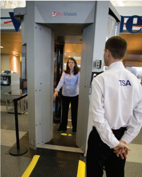
L-3’s ProVision advanced imaging technology detects concealed objects with a single two-second scan, creating a complete multidirectional view. This enables ProVision to scan 200–400 people per hour depending on the application.
