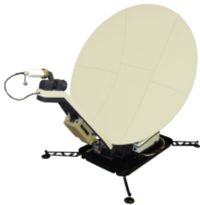
Deployed 1.2 m Antenna
