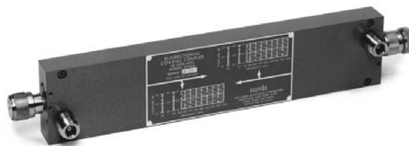
Figure 8. Coaxial Dual Directional Coupler
