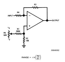
FIGURE 2. Offset Voltage Adjustment for Inverting Amplifiers Using Any Type of Feedback Element
