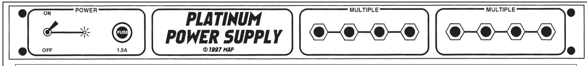
Figure 7 - The switch, LED, and fuse for the power supply fit behind a standard 1U rack panel, leaving plenty of room for two multiples.
