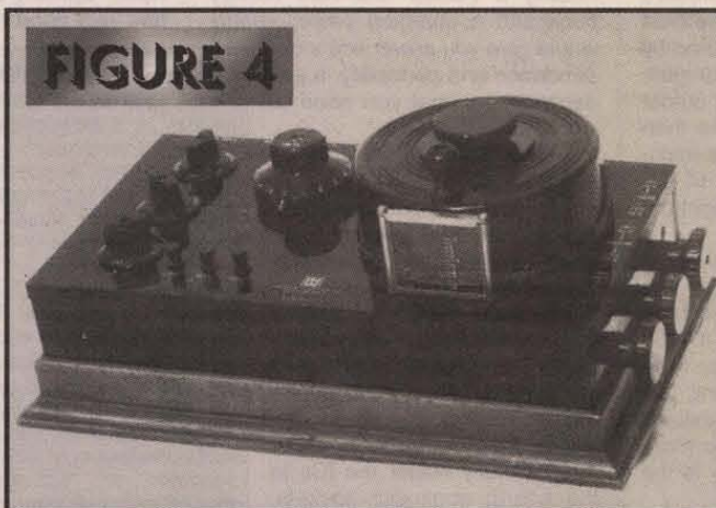
Leeds and Northrup Model 7552 is a typical potentiometer. Input and output binding posts are on rear panel (not visible). Large "drum" with crank handle is the spiral slidewire.
