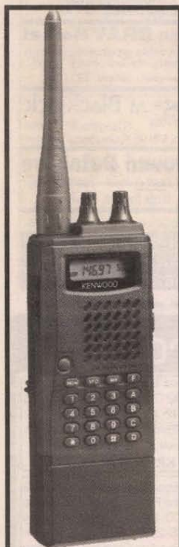
The new low-cost ham radio from Kenwood features a mike circuit that won't creep up to overdeviate when crowd noise gets loud.
