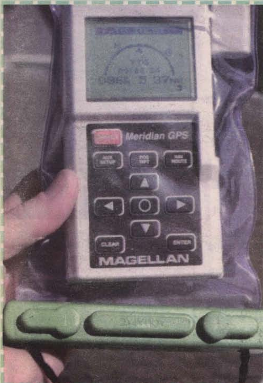
Once the bag is sealed, this GPS receiver can now go down to 30 feet under water!
