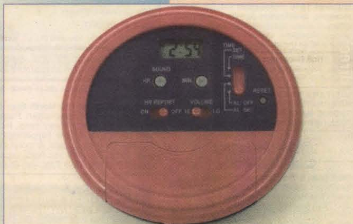
The LCD time display and all controls except the dome switch are underneath the clock.
