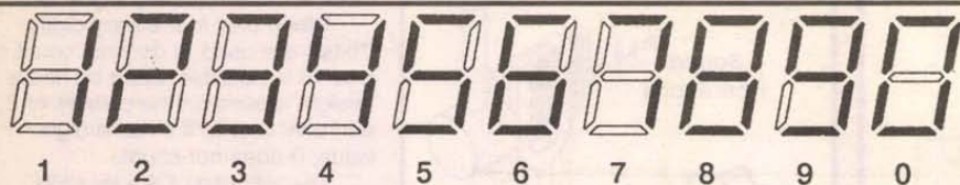
Figure 6 - All decimal numbers from 1 to 0 can be represented by seven "segments."
