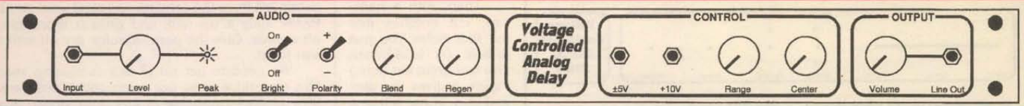
FIGURE 3: With a computer artwork or drafting program, lay out your front panel as in the example shown here. Use reasonable representations of the knobs, switches, jacks, LEDs, and so forth so that you can get a feel for the "ergonomics" of the panel. Allow plenty of finger room between the various controls.
