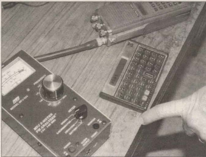
FIRST, CALCULATE FREQUENCY ERROR AT EACH END OF THE TWO-METER BAND.
