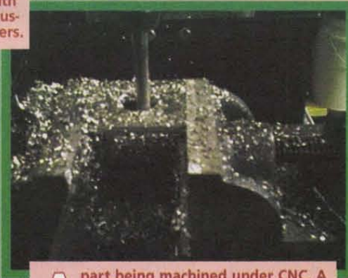
A part being machined under CNC. A one-inch hole is being circular interpolated using a 3/8-inch end mill.
