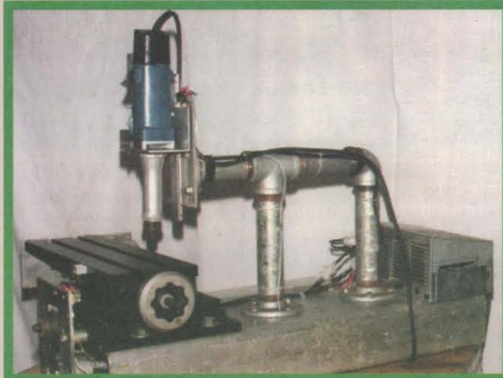
Here is another three-axis chopper driver mounted in an old computer power supply case. This CNC controller runs a modified X-Y table used for routing/engraving. The power head is a 1/4hp 25,000 RPM ball bearing die grinder.
