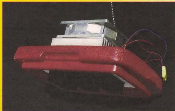
Figure 4 — Mounting the TEC assembly in the cooler lid.
