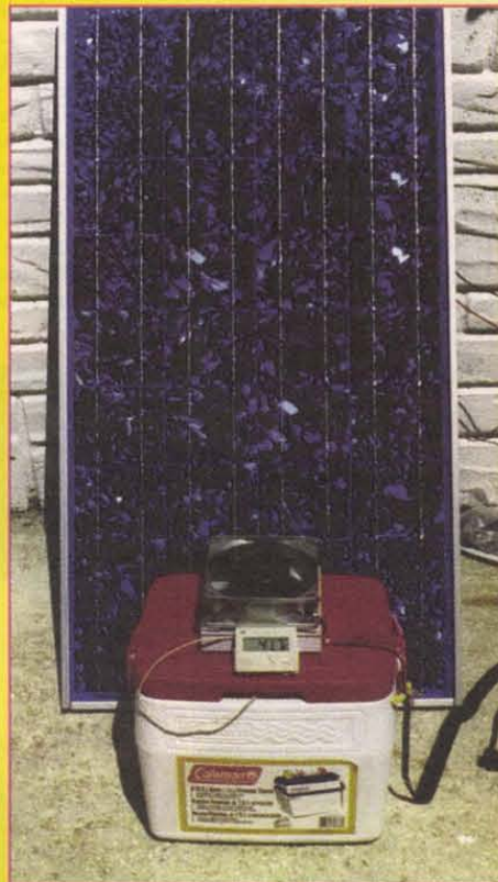
Figure 5 — Solar powering the "fridge."
