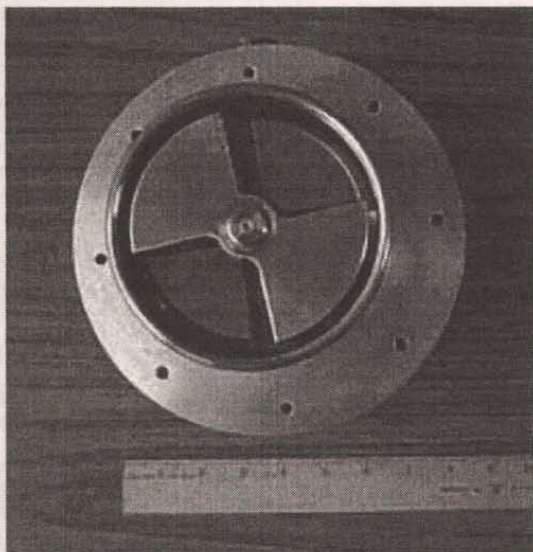
The "bowtie" rotor spins to alternately shield and expose the pie-shaped inner electrodes to the external electric field.
