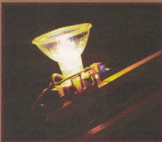
Figure 3 — 12W Halogen Mounted on Desk Lamp Arm. Switch is SPST toggle.
