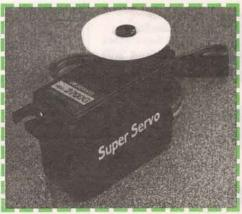
Though looking pretty much like all other servos, JR's "Super Servos" and Multiplex's MC series use a micro-processor to increase the control pulse rate, increasing power and speed.
