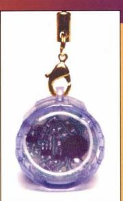
The RF Bug will sniff out and expose hidden transmitters. Place it within a few inches of the suspected item and it activates when it senses a transmission from a hidden camera or audio transmitter.
