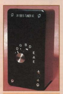
Photo B. Robbi's Tuner II Nine-note Violin/Guitar Tuner This tuner covers the ranges of both the guitar and the violin. Since it has a 12-position switch, you could expand it even more.
