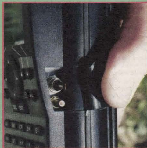
The port seen here takes the power plug for external AC or DC operation. The lower jack is for the antenna.
