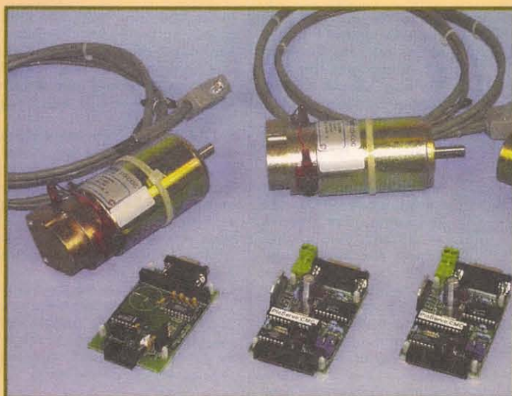
Figure 2: Motors and controllers for the CNC retrofit.
