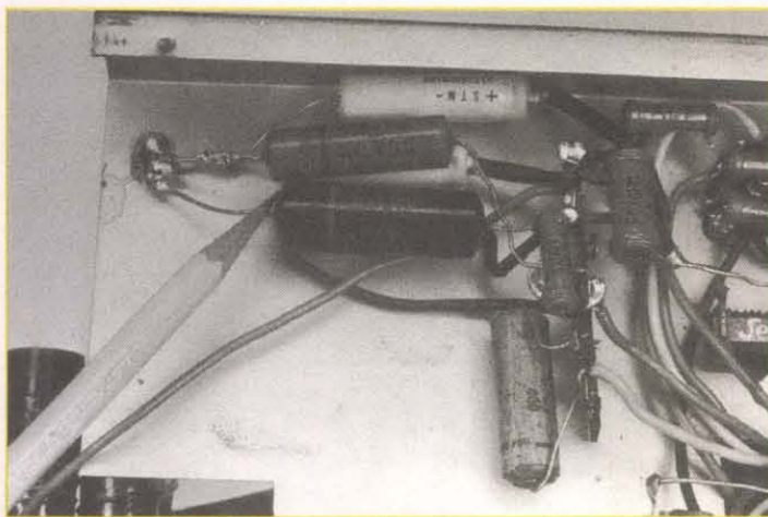
Oscillator capacitors C1 and C2 of Figure 9 were replaced.
