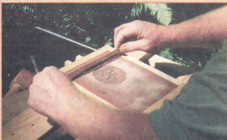
Here Gene is striking off excess sand from the drag. The pattern being molded is a medallion made especially for GEAR. The resulting casting will be awarded to the best robot built during the campout.
