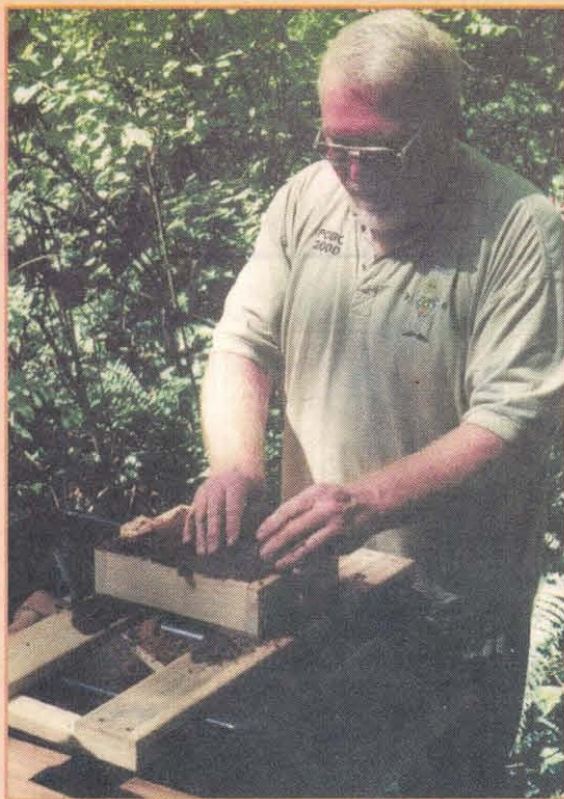
Gene Elliot is ramming up the drag half of a sand mold, the first step in the process of casting aluminum — right in the camp ground! He's using Petrobond, an oil-based casting sand that's much easier to use than ordinary "green" (moist) sand.
