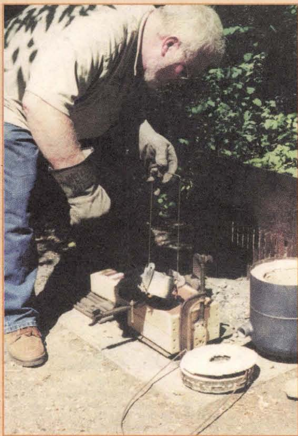
The drag and cope clamped together for the pour, Gene pours the molten aluminum from his miniature crane ladle. On the right is the home-made crucible furnace he used to melt the aluminum, and on the ground is the lid to the furnace. The stubby pipe projecting from the furnace is the tuyere, the air inlet to which is attached a hair dryer. The furnace burns nothing but plain old charcoal, and the whole setup is quieter and cleaner than any of the camp fires in the campground.
