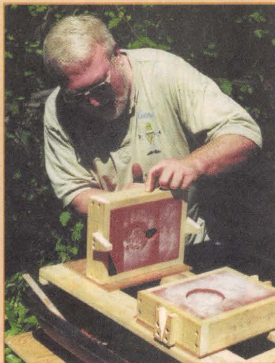
Preparing the cope half of the mold. The sprue hole has been cut, and Gene is cleaning up the pour hole on the opposite side. Note the white parting powder on the drag. The clay pattern has already been removed.
