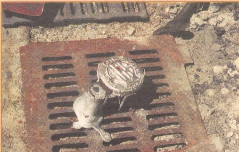
The hot casting just after shaking it out of the mold. The protruding wires on top and bottom show where vent holes were poked in the sand to allow gasses to escape while the molten metal was poured. The sprue, still attached to the left side of the medallion, provided a reservoir of liquid metal to feed the casting, keeping it from shrinking away from the mold and producing voids. With a little hacksawing and filing to remove the sprue and flashing, the medallion will be done.
