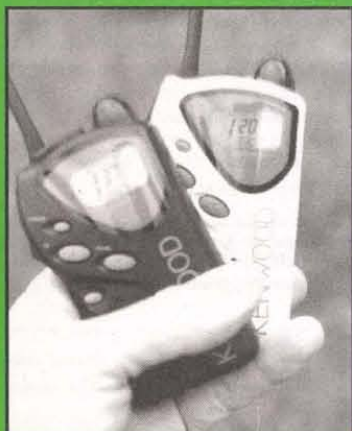
The one-half watt UHF FRS radios work up to two miles in the city.
