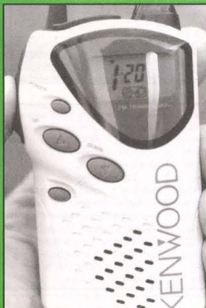
The Kenwood FRS radio has input jacks for a speaker/mike or slow scan TV.
