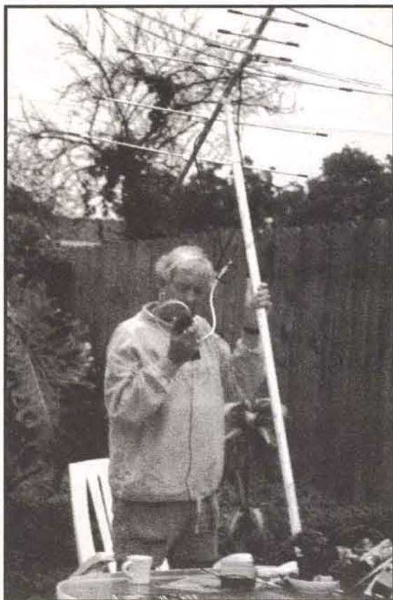
A 430 MHz beam helps pull in ATV to the portable ICOM R3 receiver.
