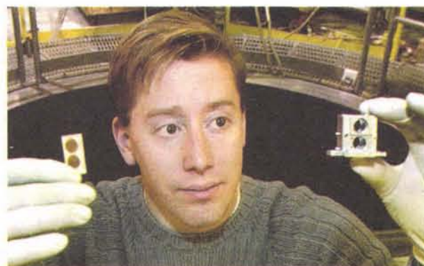
Sandia researcher Marcus Knudson holds two flyer plates in his right hand and chambers of his high-tech gun in the left. Photo by Randy Montoya.
