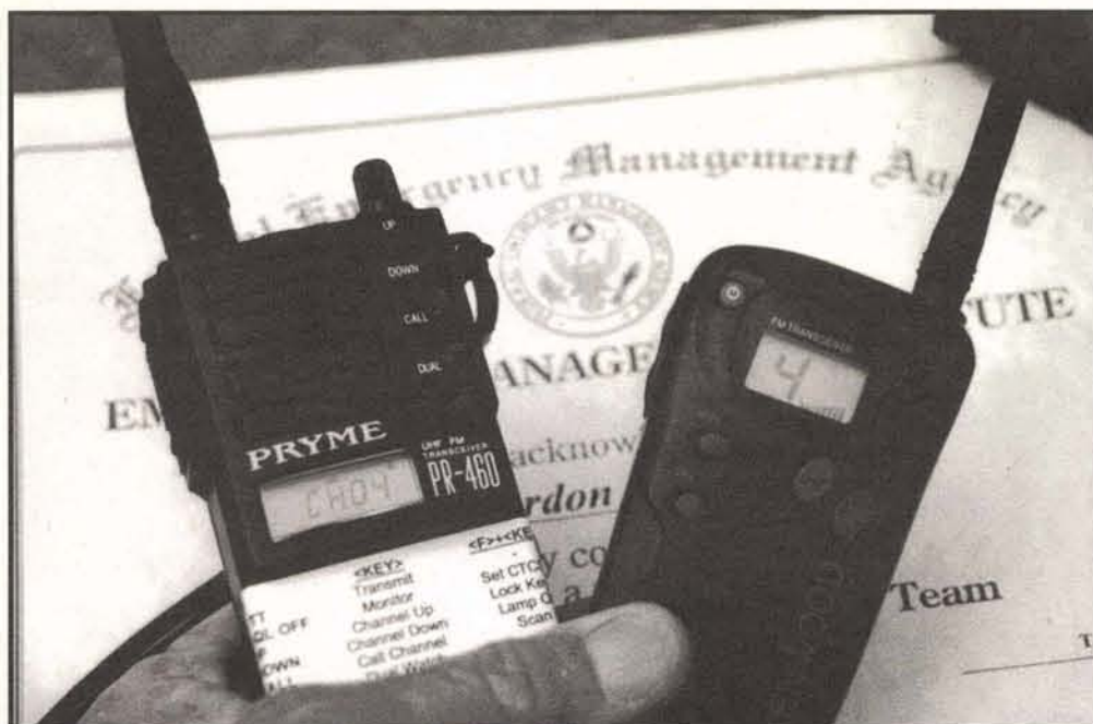
The Pryme 99 channel GMRS/FRS UHF handheld (left) and FRS radio (right) in use by CERT teams.
