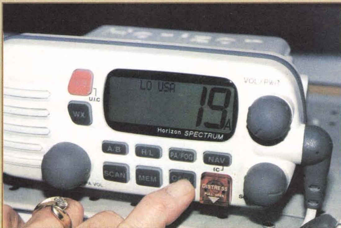
The horizon spectrum DSC VHF radio will automatically echo a position polling request.
