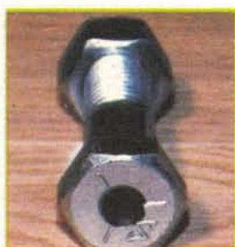
Photo 2 — Snapshot of a bolt with a 10 mm diameter hole through it.
