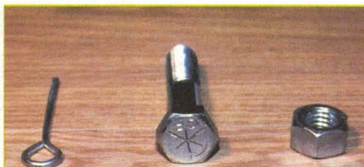
Photo 3 — Snapshot of a 5/8 x 3" bolt before it is drilled, along with the nut and the locking pin.
