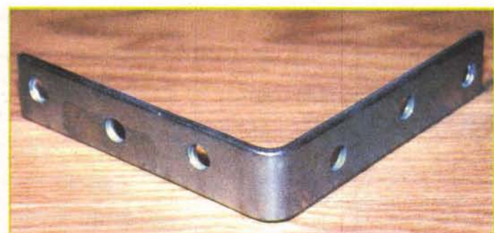
Photo 4 — Picture of one of the six-inch angled steel brackets used in making the heavy-duty motor mounts.
