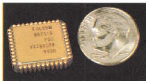
The Falcon IC is a small CMOS device that provides high-resolution time measurements. Photo courtesy of Sandia National Labs.
