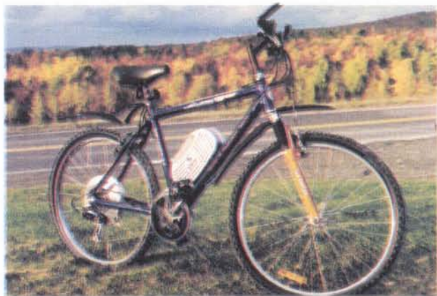
The power-assisted touring bike from EPS, Inc., provides a range of 25 to 50 km (15 to 30 mi) on a charge. Photo courtesy of EPS, Inc.
