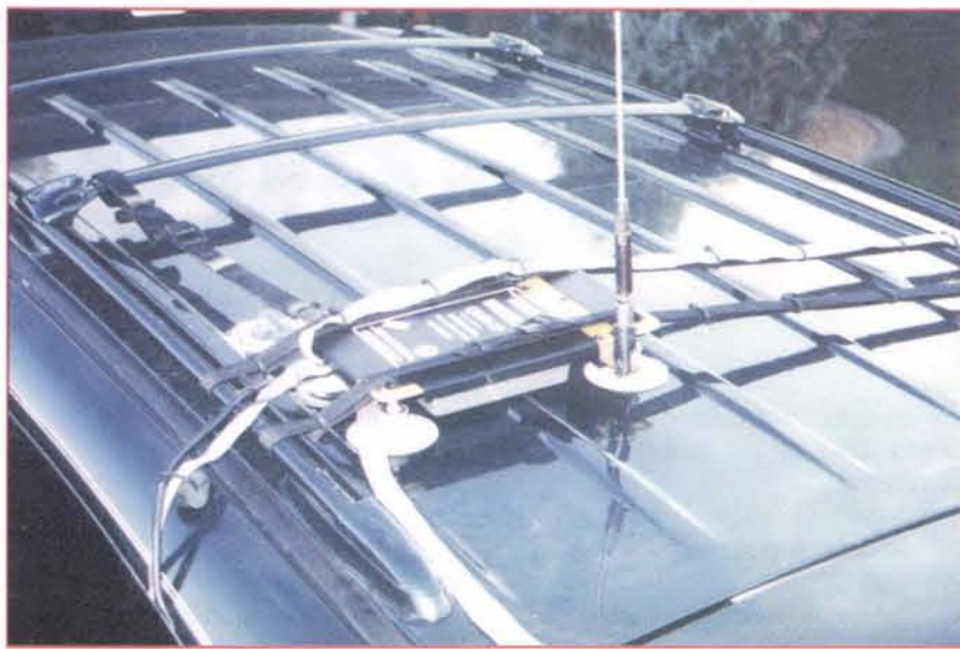
The SGC QMS system is fully waterproof for vehicle mounting on the roof.
