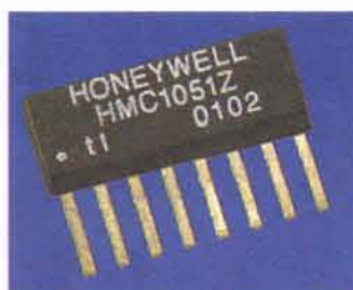
Honeywell's 1051Z single-axis magnetic sensor combines with the CMC1052 for three-axis position sensing applications. Courtesy of Honeywell Solid-State Electronics Center.
