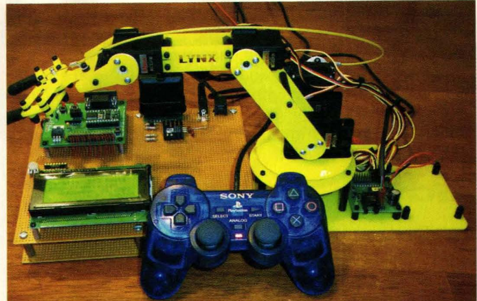
Photo 1. Complete project — Lynxmotion Lynx 5 control via Parallax BASIC Stamp with a Sony Playstation controller used as an input device.
