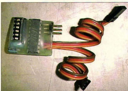
Figure 4. Ohmark brand elevon mixer. This mixer has two inputs and two outputs. It plugs in directly between the receiver and the speed controllers and mixes the signals to achieve a smooth tank drive system with a pistol grip radio. More expensive computerized radios will have this function built in. Purchased at www.planes-wings-things.com . Part# MK1.0. (Planes, Wings & Things is going out of business. You can get mixers at www.robotlogic.com .)
