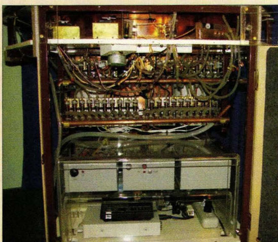
Back view. Sound module and MIDI player on the bottom, electronics above them. Rows of valves in the middle. At the top are servos for bee x-axis and ladybug, lasers for the shack, and servo for the center valve.
