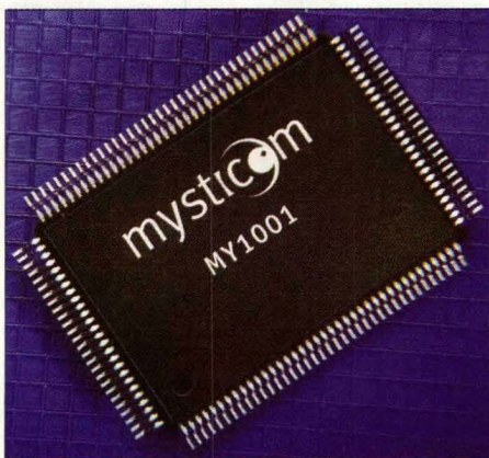
FIGURE 3. A typical Ethernet transceiver. This IC is the heart of all Ethernet interfaces. This MY1001 by Mysticom is designed to handle 10/100/1,000 Mb/s versions of Ethernet and can achieve a maximum range of 140 meters on UTP. Courtesy of Mysticom. www.Mysticom.com
