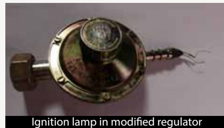
Ignition lamp in modified regulator
