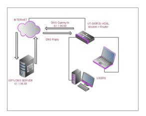
The router has a default DNS server assigned by the ISP.Some times it may be provided by a DHCP server.
