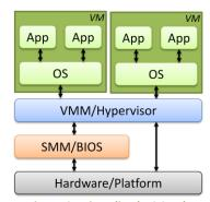
Figure 6 - Virtualized PC Stack
