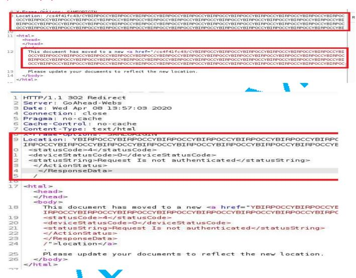
The management web interface is now disabled and the device must be rebooted to clear the condition. Thus, the device is exclusively operating as the "coolhandluke" router and legitimate web traffic is no longer being processed correctly. (Denial of Service)
