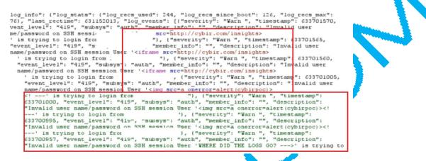
In this example, an attacker is able to inject malicious content, such as HTML or JavaScript into this log and render it in a victim's browser via specially crafted request. Final, partial PoC, injection of a valid HTML form, enabling triggering of multiple attack vectors.
