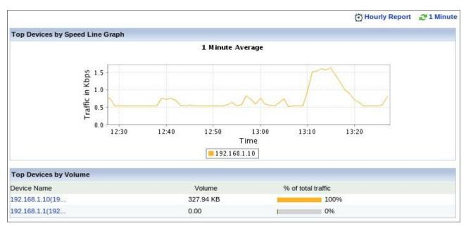
Figure 12: Capturing Start and End time of an attack using Netflow export
