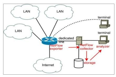
Cisco Netflow Configuration for measuring Network traffic rate
