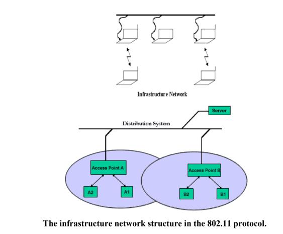
The infrastructure network has a formal structure. It uses fixed access points (AP), which are RF-enabled nodes on a hard-wired LAN. The structure allows mobile nodes to communicate with the access points to join the network. Mobile units can move freely within the area covered by the access point radios, typically a range of 100 meters for the 2.4 GHz band. The RF link is intended to operate with units moving at pedestrian or vehicular speeds.
