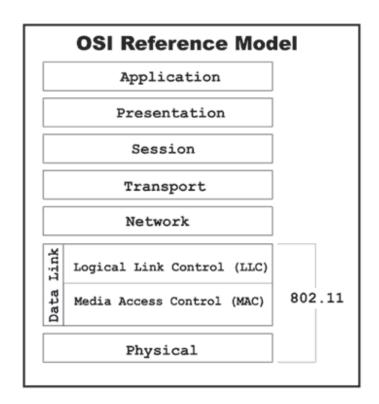
As with any of the other 802 networking standards (Ethernet, Token Ring, etc.), the 802.11 specification affects the lower layers of the OSI reference model, the Physical and Data Link layers.
