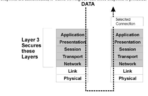
IPSec is the standard network layer security protocol, and provides a standard and extensible method to provide security to network layer (IP) and upper layer protocols such as TCP and UDP. It is used
