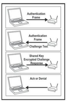
1) The wireless station begins the process by sending an authentication frame to the AP it is trying to associate with.
