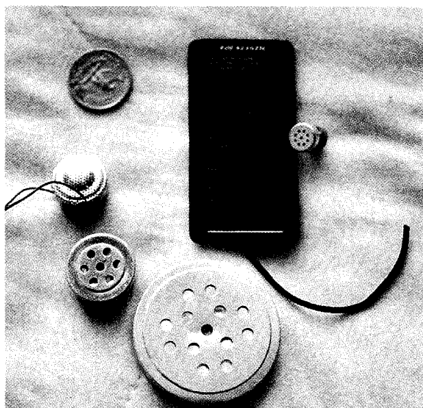
Different types of microphones. The large one on the bottom is crystal. The others are electret. They require a small electric current to work, except the square one, which is solar-powered.
