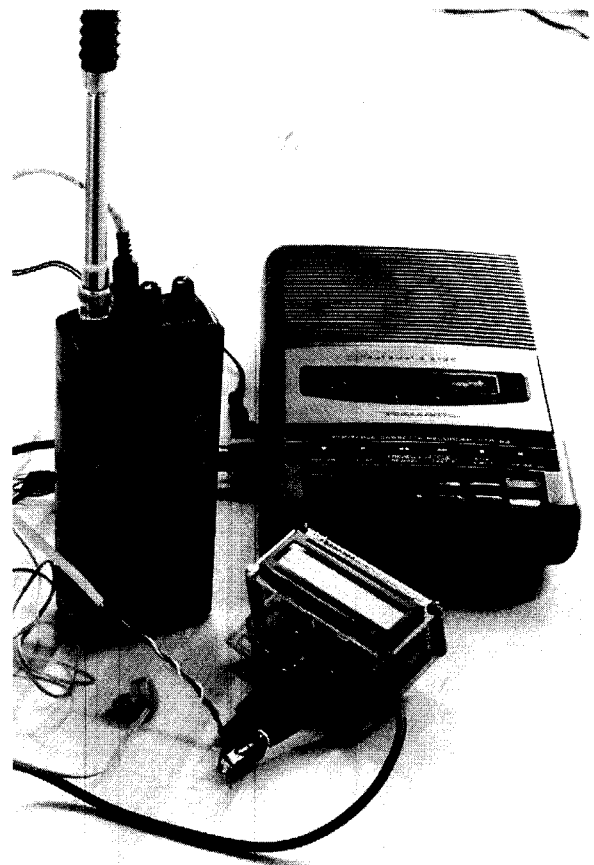
Figure 14. A homemade "Y" adapter will allow you to listen to DTMF tones while you decode them.
