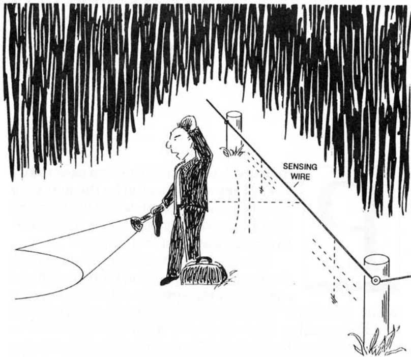
Figure 31. Proximity detector system. The intruder becomes part of the capacitive circuit of the system, which changes the input capacitance of the proximity detector.
