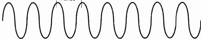
A. Unmodulated RF carrier wave
