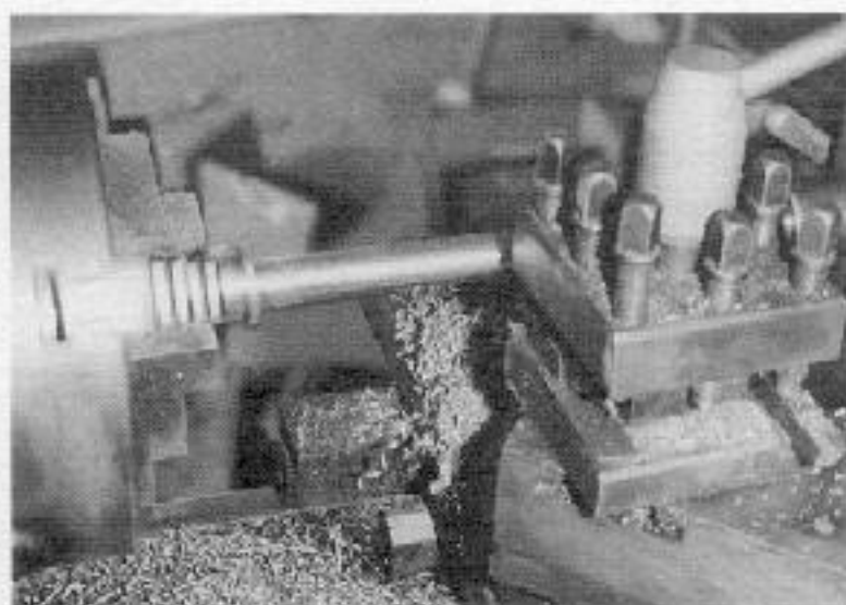
Barrel is turned to desired diameter.
