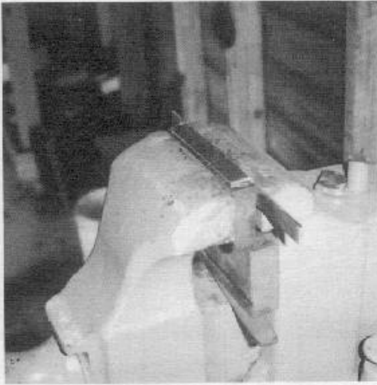
Sides are formed with block and hammer.
