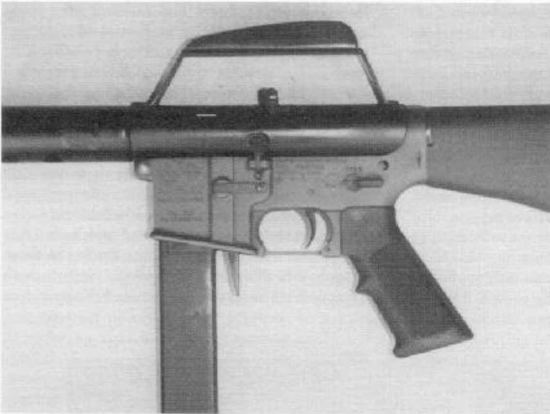
9mm conversion unit mounted on commercial receiver.
