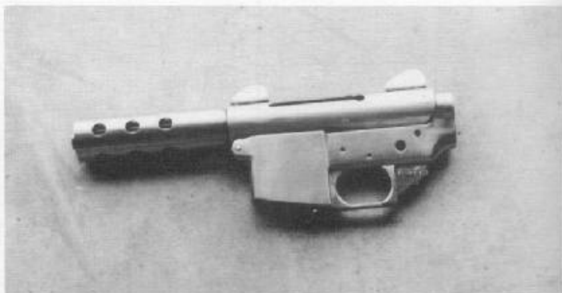
Completed lower receiver with pistol version upper pinned in place.
