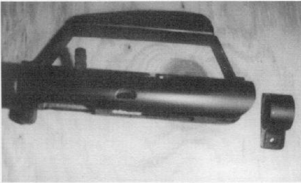
Cut near center to clear bolt release.
