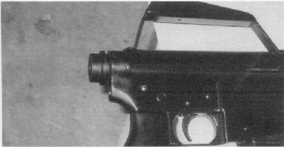
Breech plug partially screwed in place.
