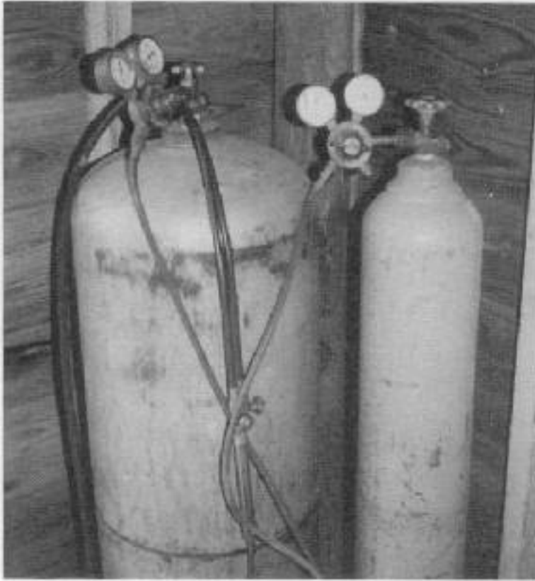
This gas welding set is used for silver-soldering, heat-treating, and coloring operations.
