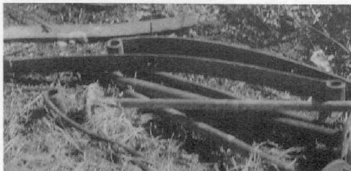
Softened steel is removed from ashes after cooling.
