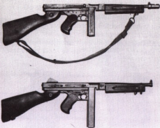
At top, a VC Thompson copy with original sling. The bottom item is the real thing. In the copy, note the imprecise cut on the cocking slot, the missing fin on the aluminum compensator, plus other assorted M1A1, M1928A1, and homemade parts. (Courtesy of Fred Rexer, Jr.)
