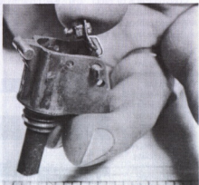
This unusual .22-caliber firing device was made by taking the detonator top from an inert grenade, drilling out the primer area, and inserting a .22 round. The firing pin is spring-loaded. (Courtesy of Oceanside, California, Police Department.)
