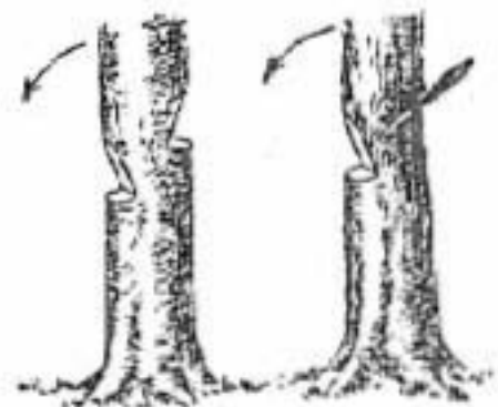
Picture 9. Notches for the Direction of Fall
