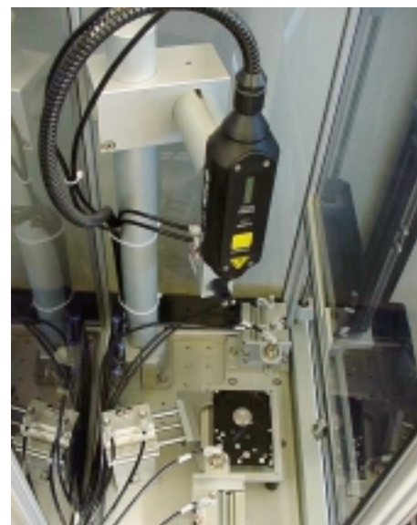
Production line test stand for checking hard disc vibrations. Photo courtesy of PMDM Germany.
