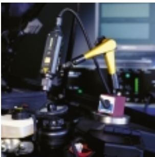
Vibration measurements on the alternator of a running engine.
