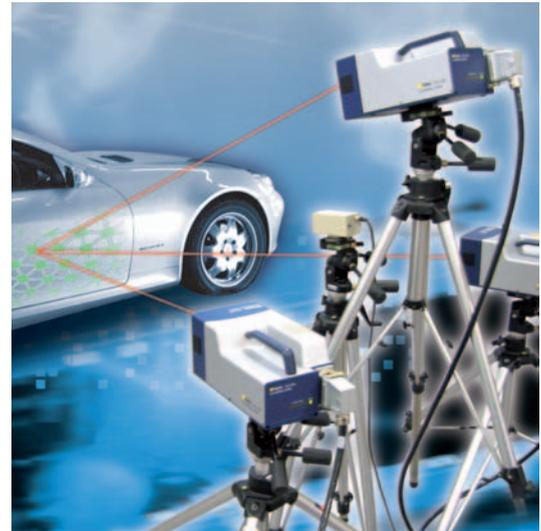
The PSV-400 Scanning Vibrometer is used to study objects of very different sizes including large automobile bodies, airplane fuselages, ship engines and buildings as well as tiny silicon micromachines, hard disk drive components and wirebonders. Demanding applications such as measurements on hot running exhausts, rotating surfaces, underwater objects, delicate structures or ultrasonic devices are all made possible by the PSV-400.
